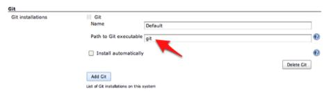
Figure 5.8. System-wide configuration of the Git plugin
