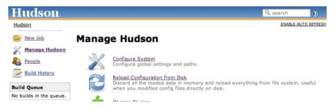
Figure 13.14. Reloading the configuration from disk
