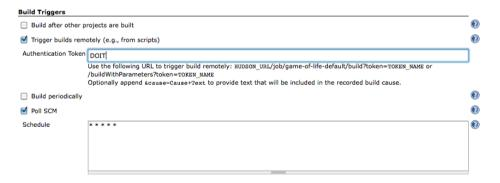
Figure 5.25. Triggering a build via a URL using a token
