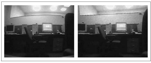
Figure 11-12. Camera image before undistortion (left) and after undistortion (right)
