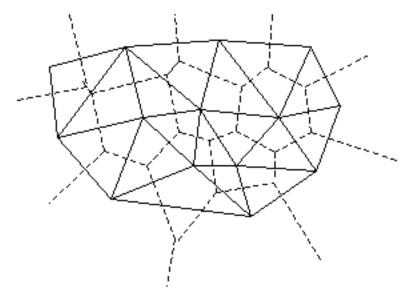
OpenCV subdivides a plane into triangles using the Delaunay's algorithm. Subdivision is built iteratively starting from a dummy triangle that includes all the subdivision points for sure. In this case, the dual subdivision is a Voronoi diagram of the input 2D point set. The subdivisions can be used for the 3D piece-wise transformation of a plane, morphing, fast location of points on the plane, building special graphs (such as NNG,RNG), and so forth.
