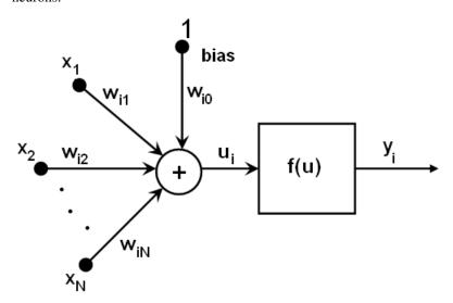
In other words, given the outputs  $x_j$  of the layer n, the outputs  $y_i$  of the layer n+1 are computed as:
