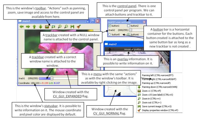
This figure explains new functionality implemented with Qt\* GUI. The new GUI provides a statusbar, a toolbar, and a control panel. The control panel can have trackbars and buttonbars attached to it. If you cannot see the control panel, press Ctrl+P or right-click any Qt window and select **Display properties window**.
